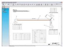
Flatten electrical cable and harness routes, detail, and generate manufacturing documentation quickly and easily.
